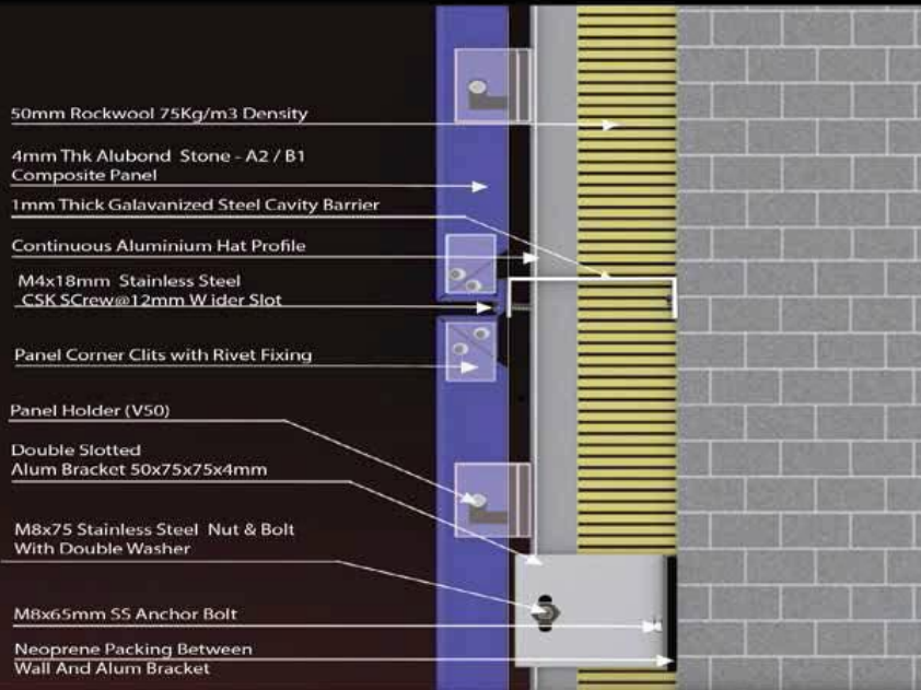
ABTI - OPEN GROOVE VENTILATED SYSTEM WITH CAVITY BARRIER EACH FLOOR TYPICAL PANEL VERTICAL FIXING DETAILS RAIN SCREEN CLADDING
