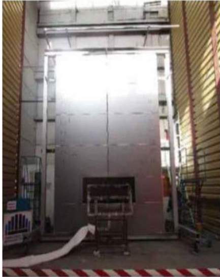
NFPA 285 PANEL FACES PRIOR TO FIRE TEST
