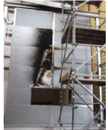
WALL CAVITY IN WALL ASSEMBLY AFTER FIRE TEST
