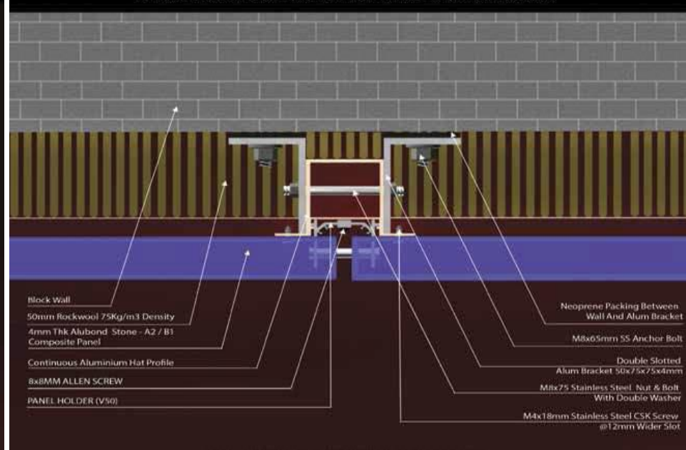
ABTI - OPEN GROOVE VENTILATED SYSTEM TYPICAL HORIZONTAL FIXING DETAILS RAIN SCREEN CLADDING
